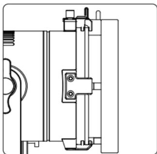
Make sure the pick is pushed to the front of the claw before installation.
