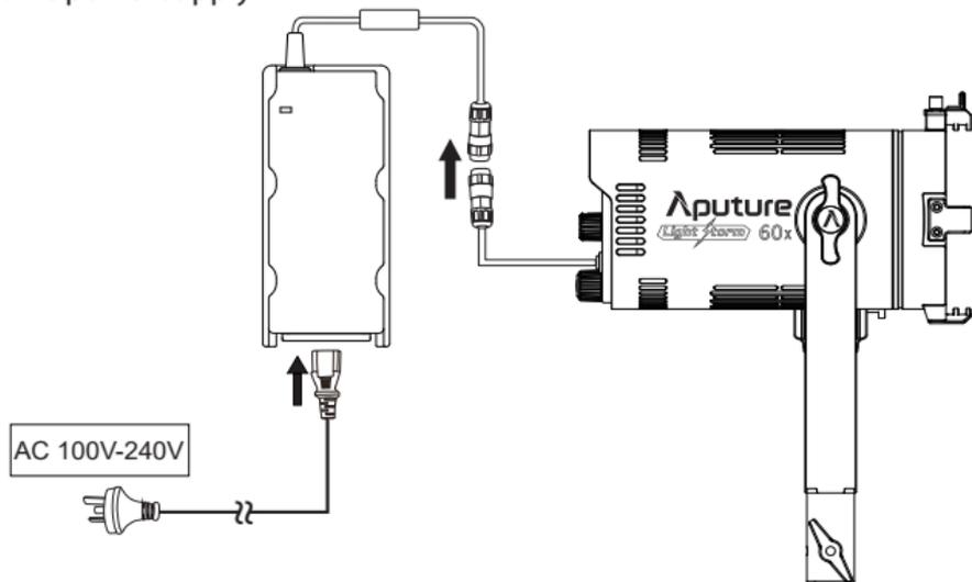
\* Rotate the red rotary ring of the DC input connector clockwise, then pull out to remove the adapter.
