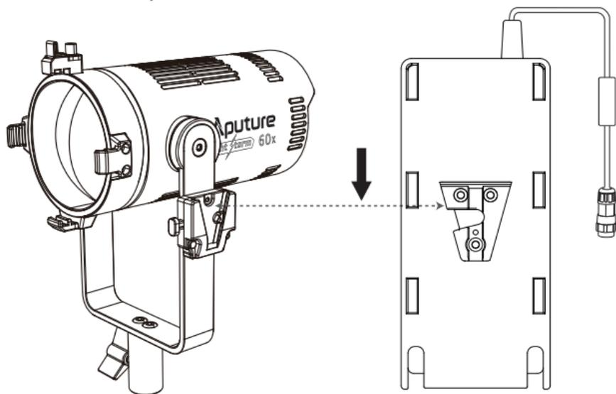
*\* To remove the Adapter, press the V-mount seat button and pull the Adapter case upward.*
