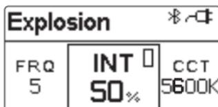
\* In explosion mode, short press the Trigger button to single trigger the light effect.
