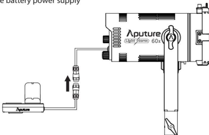
\* When using a single battery for power supply, be sure to install the battery in the battery slot corresponding to the red key; When removing the battery, press the red lock button to pull out the battery. Do not hard pull out.
